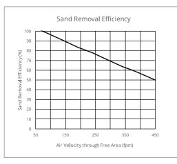
Sand removal efficiency approximately 90%, measured during tests described in ASHRAE Standard 52-76 test method.
