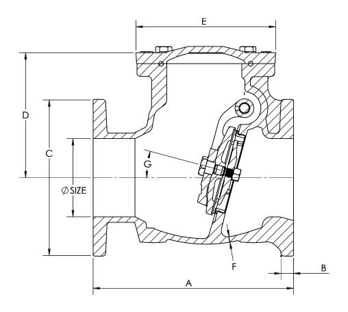
FIGURE 1126 & 1126A STANDARD DIMENSIONS WEIGHT
