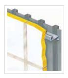
As an alternative to the above, timber packing strips may be cut to suit the sheeting rails and screwed in place, fix the KBR at the head of the wall by screws into the timber packer with a steel strip placed on top of the insulation directly over the packer. Repeat as required at other sheeting rail locations, ensuring that the KBR are closely butted to each other with the edge flanges overlapping.
