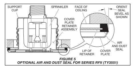
Step 7. When installing an Air and Dust Seal, see Figure 5; otherwise, proceed to Step 8. To attach the Air and Dust Seal, verify the angle of the outside edge of the seal is oriented according to Figure 5. Start the edge of the Retainer in the grooved slot of the Air and Dust Seal and continue around the retainer until the entire Air and Dust Seal is engaged.
